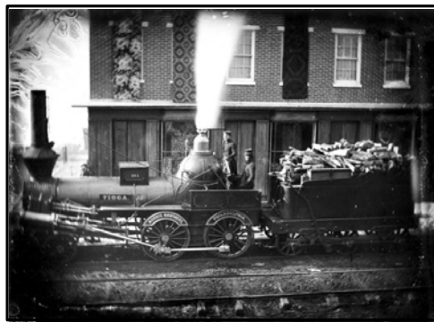
The Norris Bros. 1848 built Tioga illustrates the open and primitive conditions early engineers faced. It took only one winter to convince resourceful shop employees to build improvised cabins to stay warm. Later term for the vehicle driving area would be abbreviated to cab.
