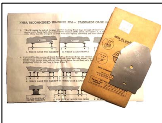
The NMRA HO track gauge is a multi-faceted tool which provides verification of wheel set dimensions, switch dimensions, platform/side clearances, and flangeways. Instructions illustrate how the gage is used.
