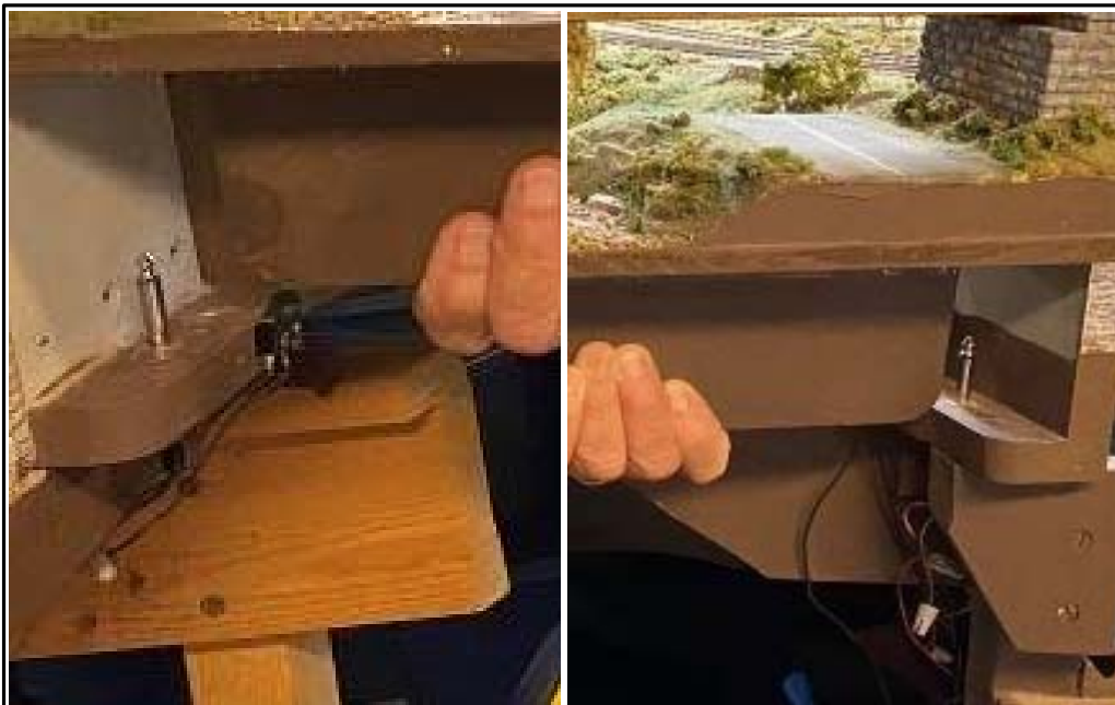
A completed bridge spans the aisle way to the center of the layout. The bridge section lifts out if needed. Note the alignment pins and electrical switch at bottom left which cuts power to the track approaches.
