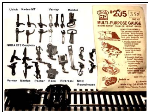
The NMRA XF2 'horn hook' coupler brought commonality and functionality to a standard less hobby. Couplers could mate and release hands-free regardless of manufacturer.
